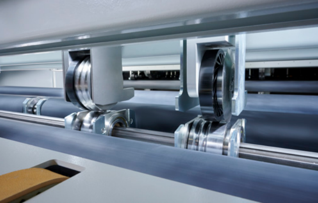
Crease standard, Bottom Crease and Line Cut
